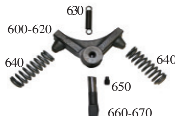
600. Angle pawl - dia. of shaft 20mm up to chassis No. 737. 610. Angle pawl - dia. of shaft 22mm up to chassis No. 1508. 620. Angle pawl - dia. of shaft 26mm from chassis No. 1509 - 630. Anchor spring for angle pawl.
